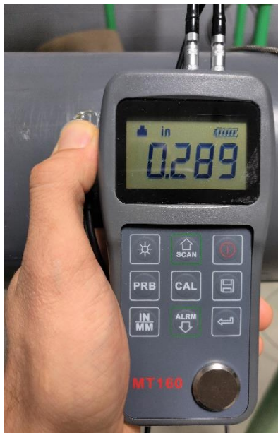
Figure 8: Measuring Wall Thickness of a PVC Pipe
