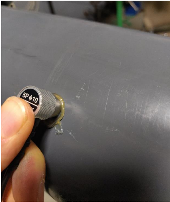
Figure 7: Transducer Being Pressed into Couplant on Pipe
