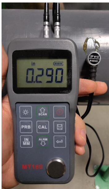
Figure 9: Drawing Out the Couplant in Scan Mode
